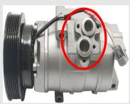
Visually check the positioning of the pipe fitting
