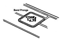
BEND THE 2 PRONGS OF THE LOWER RESTRICTOR HALF OUTWARD over the outer edge of the upper restrictor half using a blunt tool. Make certain the prongs are pressed down tightly so that the restrictor assembly is held securely in the gasket body. Turn the gasket over and repeat the prong bending operation with the other restrictor half.
