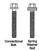
The gasket(s) included in this set will function with manifolds having either "Conventional" or "Spring Washer" style bolts.
