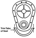
ATTACH AND ALIGN GASKET: Apply a quick-drying adhesive sparingly in several places on the engine casting or block. Attach gasket(s) on surface where adhesive was applied. Allow time for adhesive to set. Test for slippage with light pressure. If gasket moves, allow more time.
