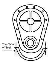
**ATTACH AND ALIGN GASKET:** Apply a quick-drying adhesive sparingly in several places on the engine casting or block. Attach gasket(s) on surface where adhesive was applied. **Allow time for adhesive to set.** Test for slippage with light pressure. If gasket moves, allow more time.
