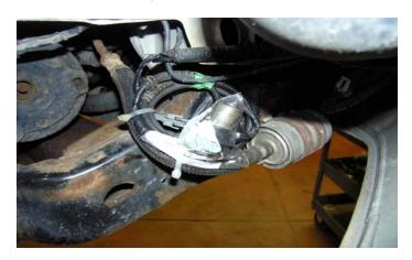
FIG 6, Solenoid Removal on Rear Shock
