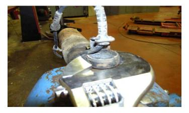
FIG 7, Rear Shock Solenoid Removed
