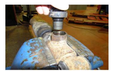
FIG 8, Solenoid Package Tucked in Frame
