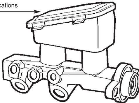
**Caution** If two different brake fluids have been mixed, the brake system should be flushed, and fresh brake fluid recommended by the vehicle's manufacturer should be installed.
