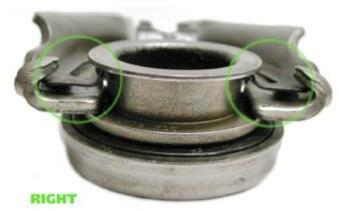
The clutch release fork spring tabs must be installed under the rear flange of the bearing, never behind the rear flange. Incorrectly installed will cause:
