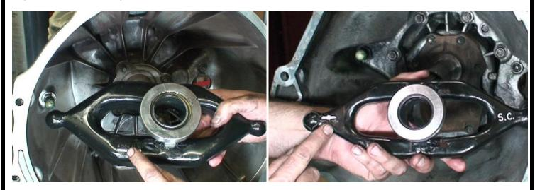
Cast iron bearing collars require grease in the collar grease groove and a light film on the guide tube. A daub of grease should also be applied to the release bearing collar fork ears.
