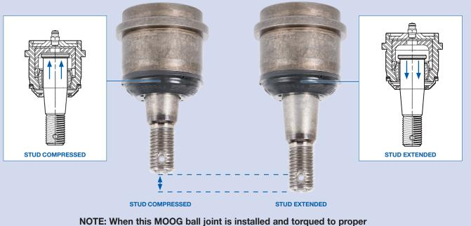
specifications, it automatically adjusts to the required extended length.
