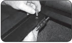
B. Push cover bar forward until it sets flat on front of side rails and overhangs them. Slide left tension adjuster over until it engages under front of side rail. Push bar back and forth to line up holes—do not turn dial wheel. Insert bolt from top and flat washer and nut from bottom.
