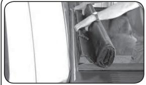
A. Set rolled up cover on rails at front of box (behind cab) with bar facing up. Roll cover bar onto front of rails and fold/tuck vinyl flap under. Now bar will face down. Let straps hang to inside of box.
