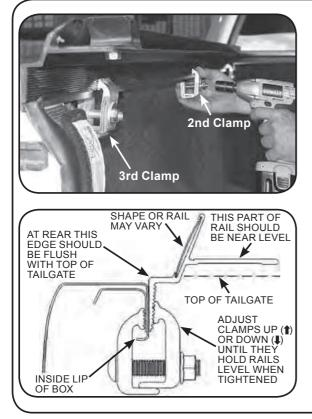
C. Install 2nd clamp on rail at midway point of box and rail. Check if rail is level. Install 3rd clamp as close to tailgate as possible. If rail tilts up, loosen clamp, lower it and tighten. If rail tilts down, loosen clamp, raise it and tighten.
