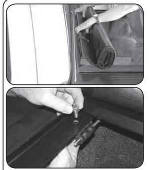
A. Set rolled up cover on rails at front of box (behind cab) with bar facing up. Roll cover bar onto front of rails and fold/tuck vinyl flap under. Now bar will face down. Let straps hang to inside of box.
