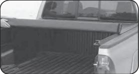
A. Unroll cover and place rear bar into strikes on side rails and press down on bar to close (20-30 pounds pressure).
