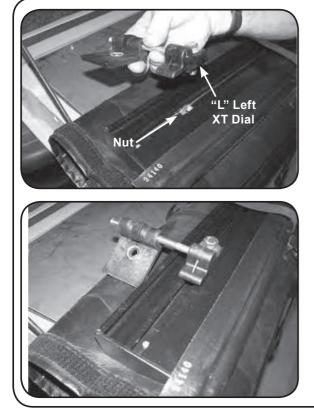
A. The cover comes pre-rolled to its normal open position for ease of installation. Set pre-rolled cover on tailgate with front bar facing up as shown. Align EZ-Dial Tension Adjuster (marked "L") on driver side of cover– positioned as shown in photo at left.
