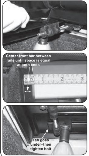
C. Hold bolt at top and tighten nut under side rail. Repeat procedure for right hand tension adjuster.
