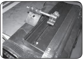
B. Turn 1-1/4" bolt with flat washer onto nut in bar. Leave loose for now. *See photo.* Repeat for EZ-Dial ("R") on passenger side of cover, and leave that bolt loose also.
