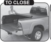
Release retainer straps at front and using both hands roll cover out to rear of box.
