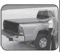
Now along side of box, seal cover edges with hook and loop sealing system the full length of cover on both sides. Pull with one hand seal with other hand.
