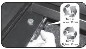
C. Check cover tension by releasing autolatch and open and close rear bar several times. It should snap down when closing. Cover fabric should sounds drumlike when tapped on. If adjustment is needed, roll cover open and turn EZ-Dial counter-clockwise to tighten, clockwise to loosen. Always turn dials in equal amounts.
