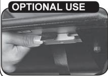
Manual Slide Lock (use is optional) is located under cover bar on passenger side push slide lock to engage, pull to disengage.
