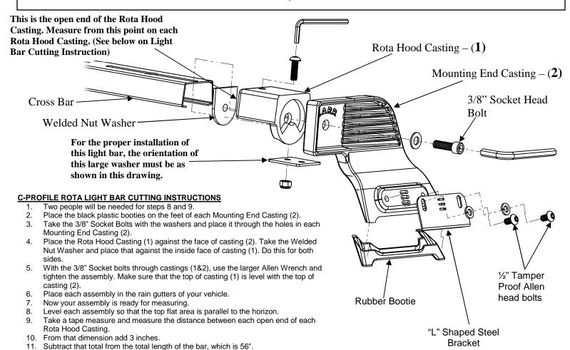
**MATERIALS NEEDED:** Hammer, center punch, pencil. (Possible drill motor with a 3/8" drill bit)
