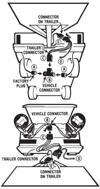
NOTE: To increase the service life of and prevent damage to the assembled system, secure it to your vehicle with cable ties or electrical tape.
