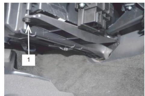
Install the cover plate hook onto the insert of the HVAC module and then press the cover plate flush.
