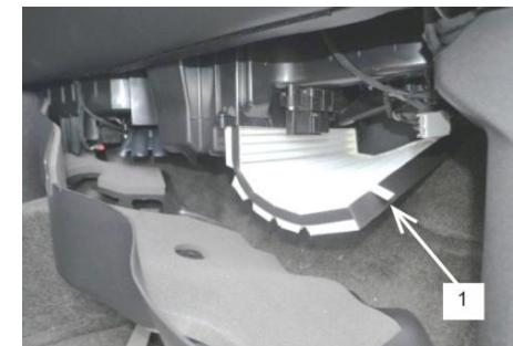
Insert the cabin air filter into the HVAC module with the pull strip (1) pointed downward. The filter stages (cut outs) are to face inboard.
