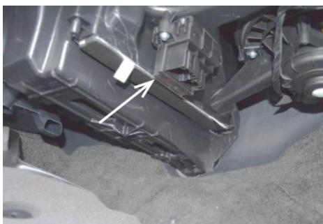
The cabin air filter needs to be flush with HVAC module access opening.
