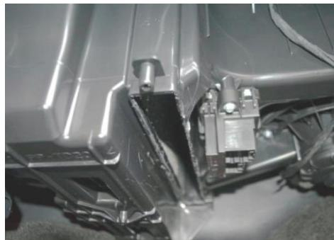
Carefully cut out the cabin filter access panel using a suitable tool. Keep the tool inside the groove at all times.
