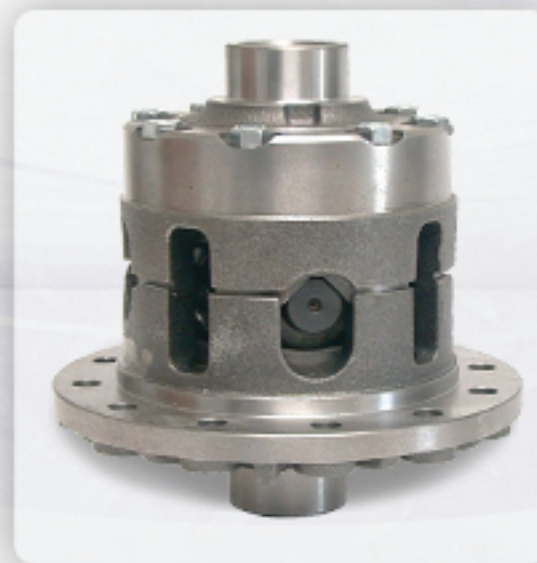
Dana Spicer Factory Positraction, "Powr-Lok". Two piece case that bolts together and has four pinion gears.
