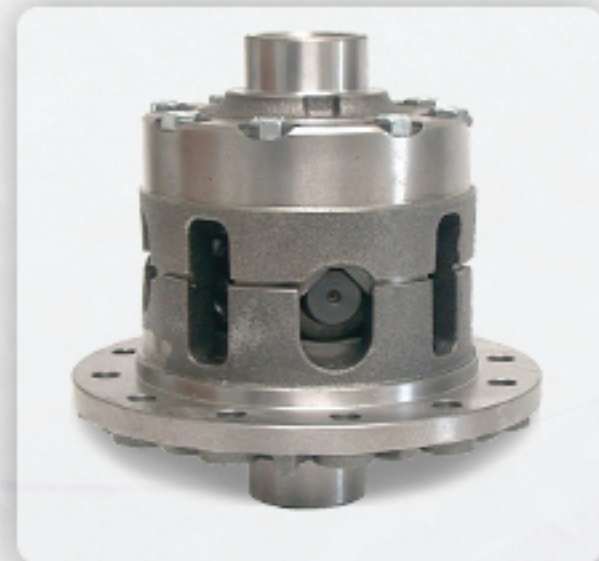
Dana Spicer Factory Positraction, "Powr-Lok". Two piece case that bolts together and has four pinion gears.
