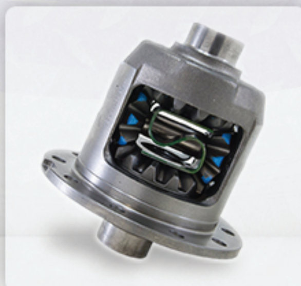
Ford Factory Positraction, "Trac-Loc". Has a S-shaped spring in between the spider gears (which you can see colored green in this photo) and has clutches located behind the spider gears.
