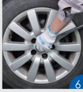
Tighten the axle nut and wheel bolts.
