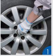
Loosen the nut from the axles and wheel lugs.
