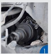
Put the flange type joints into the differential gear and install gaskets and bolts, then lock with special tool.
