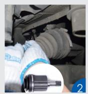
Put inner joint with circlip groove into the differential gear. Note: After installation, please try to pull out to make sure the circlip is locking into the right position in the gear
