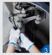
Loosen the suspension parts: Struts, ball joint control arm, etc. whichever is necessary to remove the axle or CV Joint.
