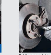
Put the outer joint into the wheel hub with washer and bolt and lock with a special tool.
