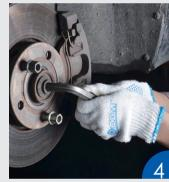
Remove the nut/bolt from the outer joint of wheel hub.
