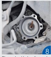
Clean wheel hub spline and the inner spline of differential gear to make sure there is no dirt or contaminants. Note: Check the wheel hub spline & oil seal of differential gear to see whether they are
