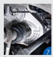
Most inner joint design plug into the gear and use a circlip internally to keep them from sliding out, to remove use a pry bar between the differential housing and inner housing to "pop- out " the inner joint.
