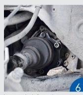
Loosen bolt from the differential gear and remove the flange type joint. (if inner joint has bolts)
