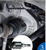
Put inner joint without circlip groove into differential gear, and please check whether they are installed correctly or not.
