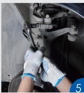
Tighten suspension connection: Ball joints, control arms, struts, etc.
