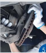
Separate joint from wheel hub.
