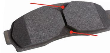
**Purpose:** The V-chamfer reduces high vibration from the center of the disc brake pad. V-chamfer is typically used in combination with parallel or radial chamfers.
