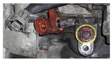
Clear debris, old O-rings, broken sensor remains, and grease:
