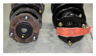
On some vehicle applications, the upper mount can be rotated freely. In this case, insert the studs at the top of the strut assembly in the car's mounting holes before installing/tightening any mounting hardware at the bottom of the strut.
