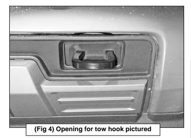
Remove the bolts securing the driver side of the bumper to the bumper bracket. Use a large screwdriver or pry bar to move the mounting tab up enough to get the long bolt through the tow hook out of the end of the frame
