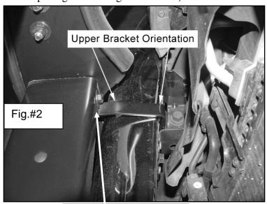
1pc M10 x 1" Hex Bolts 2pcs 10mm Oversized Flat Washer 1pc 10mm Lock Washer 1pc M10 Hex Nuts
