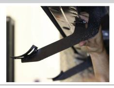
Place the side bar onto the mounting brackets and align the mounting points.
